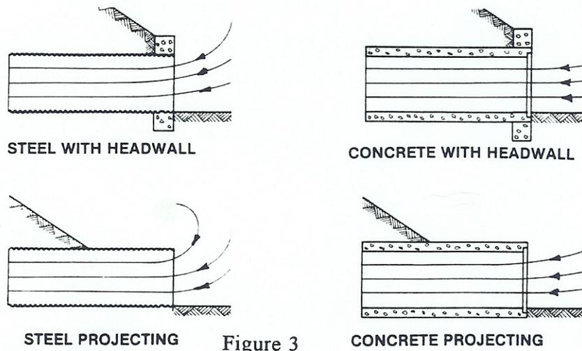
Applied coatings (bituminous, asphaltic, etc.) do not improve the hydraulic characteristics of corrugated steel pipe. According to a Missouri DOT Durability Report, *"coatings such as bituminous or polymer materials cannot be used to lower the coefficient of roughness for CMP because the coating will be lost first, leaving the hydraulic conditions controlled by the uncoated CMP."*<sup>(9)</sup>
