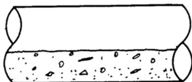
Velocity 2 fps. Efficient solids transport no sulfide buildup in small flows, up to 2 cfs. Sulfide buildup often observed in larger flows, but only at a very slow rate.
