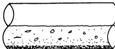
Velocity 1.5 to 2.0 fps. Inorganic grit accumulating in the bottom. More sulfide buildup as the velocity diminishes.
