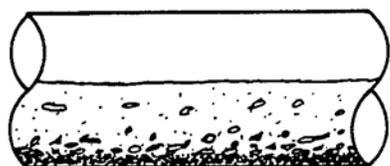
Velocity 1.0 to 1.4 fps. Inorganic grit in the bottom, organic solids slowly moving along the bottom. Strongly enhanced sulfide buildup; severe problems expected.
