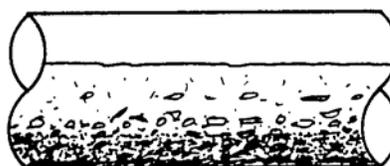
Velocity below 1.0 fps. Much organic and inorganic solid matter accumulating, overlain with slow-moving organic solids. Sulfide problems worse than in C.
